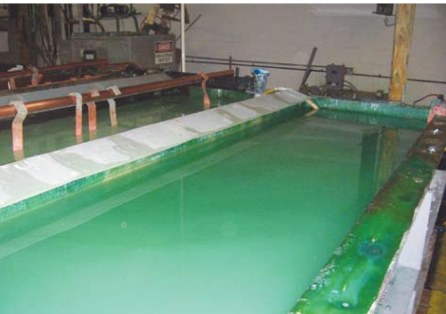
One of two, 900-gallon rinse tanks after more than 760 hr of production. Use of filtration and sodium hydroxide to normalize pH eliminates wastewater discharge.
